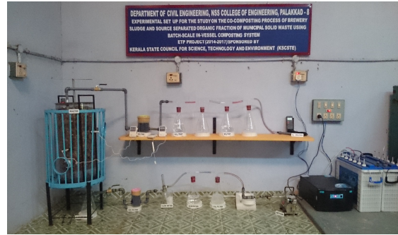
Fig 2: In-vessel reactor for lab-scale composting studies
